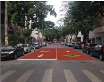
Figure 3: Horizontal signaling for the Fahrradstraße
